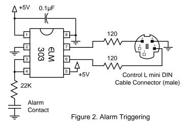
camcorder, and the camcorder is powered and placed in the camera / standby state. The cable between the two is then connected and approximately one minute later, the camera will record one sequence, and will power down. After the duration set by the Interval pins, recording will be initiated again.
